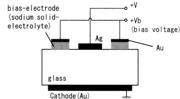
Fig.1 Schematic diagram of multi-electrode field assisted ion exchange process
