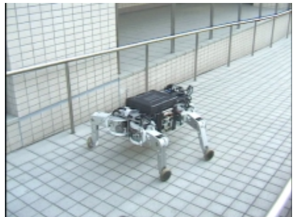
Fig.5 Slope climbing experiment
