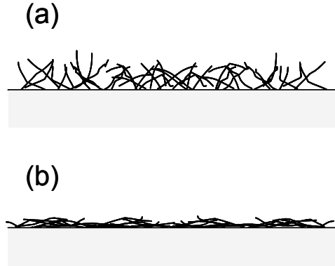
Fig. 3-17. Schematic descriptions of (a) 3D-wise and (b) 2D-wise random morphology of the SWNT films grown on quartz substrates.
