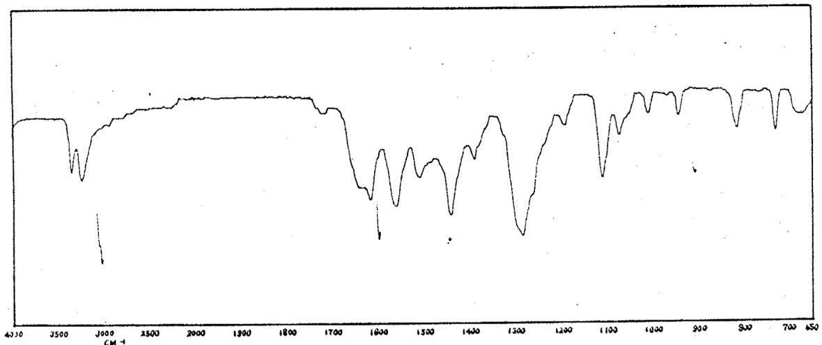
Fig 4-2 2-N-Carbomethoxyamido-3-imino-5-methylthio-TDZ
