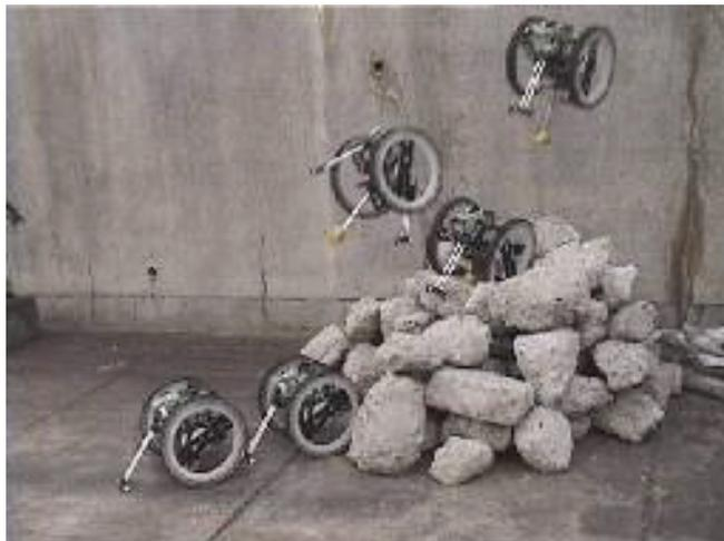
**Fig.2-9 Jumping motion of the L-in-R**
