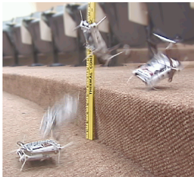
Fig.2-8 Jumping motion of the mini Whegs
