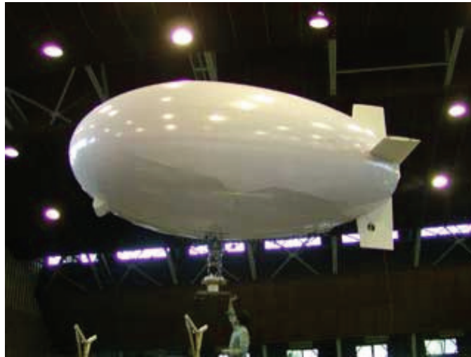
Fig.2-1 Autonomous airship for rescue
