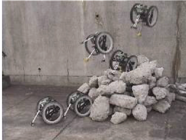
Fig.2-9 Jumping motion of the L-in-R
