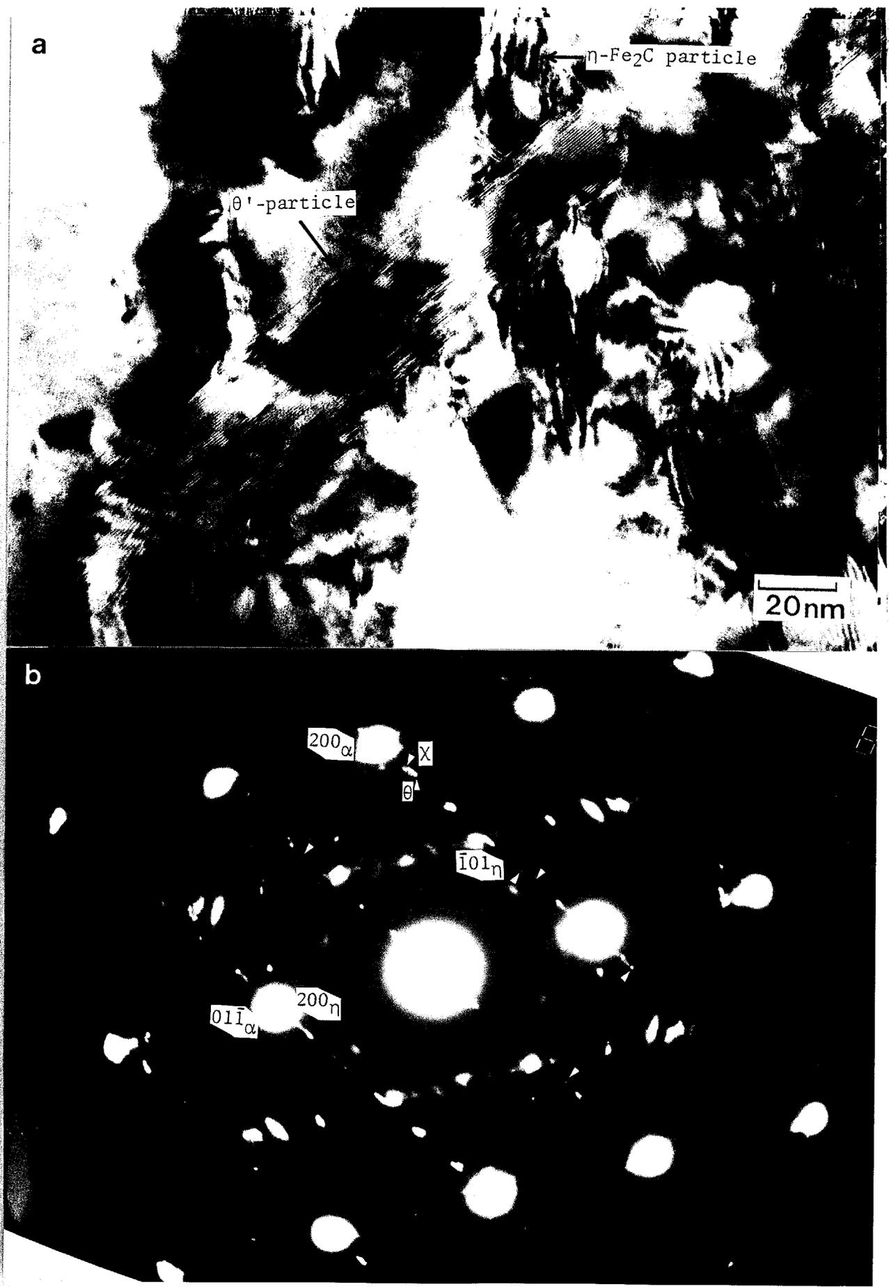
Fig. 5-5. (a) High resolution lattice image of  $\theta'$ -particle precipitated in a specimen tempered at 470 K for 50 hr.
