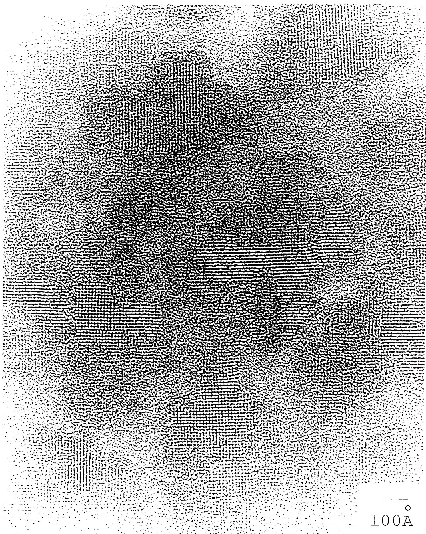
FIG. 3.7. The TEM lattice image of 100-Å (\text{AlPcF})_n/\text{KBr} deposited at -170^\circ\text{C} , then annealed at 200^\circ\text{C} , 2 h.
