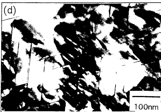
Fig.7.8 Variations of hardness with aging time for 463K aging (a) and electron micrographs and precipitate size distributions for (Mg+Ag)-added alloys aged at 463K for 36ks after W.Q. treatment from 778K (b,c) and S.Q. treatment from 673K (d,e).
