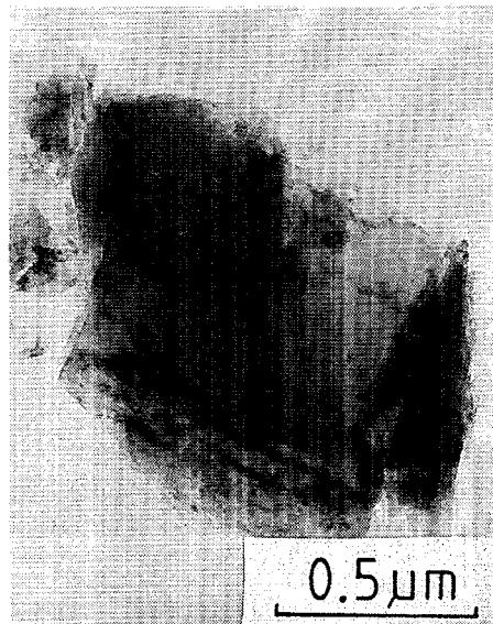
Fig.4-21 TEM observation of 10wt% CoO-doped polycrystalline MgO.
