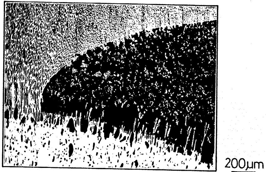
Fig. 5.22 Aggregation of L<sub>2</sub> phase at the peripherical edge of the growth front.
