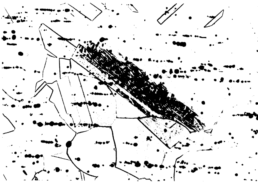
Fig. 3-7, Optical micrograph of \alpha -martensite in a polycrystal, of which average grain diameter is 28\mu revealed by polishing and etching.
