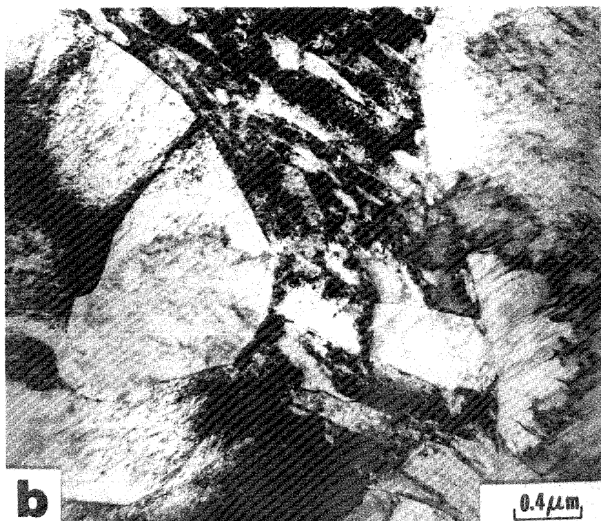
Fig. 4-14 Transmission electron micrographs of the alloy partially transformed at 600^{\circ}\text{C} for 85 sec.
