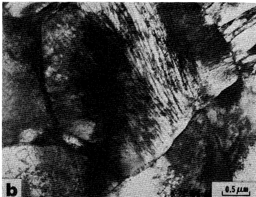
ig. 4-9 Transmission electron micrographs of the alloy partially transformed at 710°C for 85 sec.
