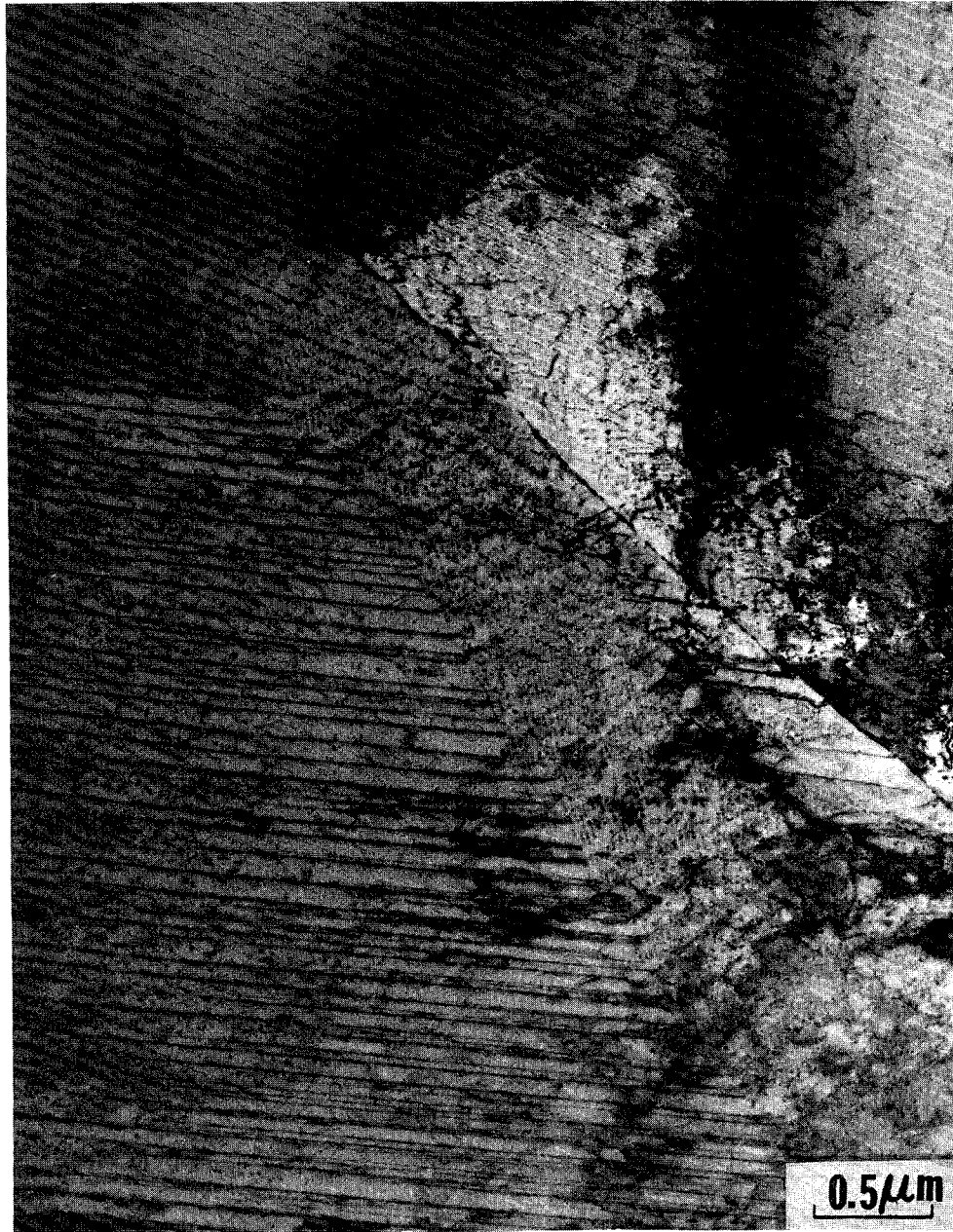
Fig.5-6 VC morphology in ferrite in Fe-0.2%C-1%V-1.5%Ni alloy isothermally transformed at 625°C, below the nose of the C-curve, for 1 hour.
