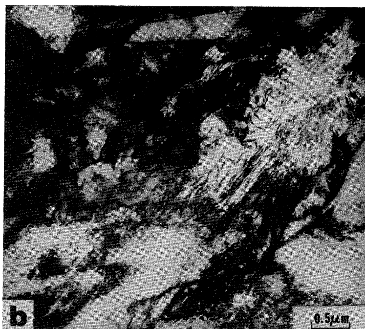
4-16 Transmission electron micrographs of the alloy completely transformed at 600°C for 420 sec.
