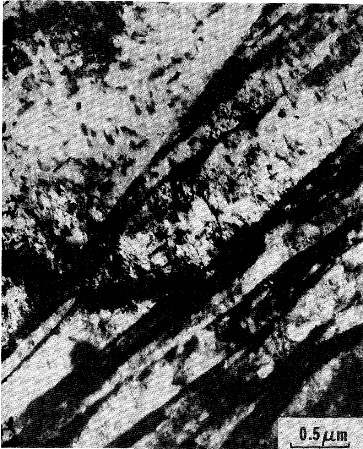
Figure 2-12 Transmission electron micrographs of Alloy 3 ausaged at 700°C for 1 hour. a) Bright field image b) Dark field image of VC c) Dark field image of Fe 3 C.
