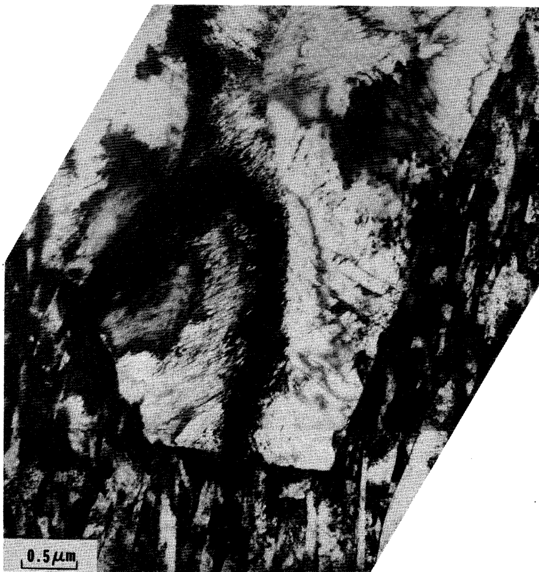
ig. 4-15 Composite transmission electron micrograph of the alloy partially transformed at 600°C for 85 sec.
