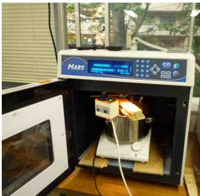
Figure 5.3 Photo of extraction using oil bath.
