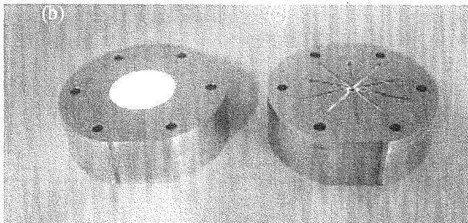
Fig.1-8 Photographs of catalytic wall microreactor. (a) Assembled device; (b)catalyst plate (catalyst size =  $\phi 32.0$  mm (diameter)  $\times$  0.5 mm (thickness)); (c)microchannel plate (channel size = 0.8 mm (height)  $\times$  1.0 mm (width)  $\times$  16.0 mm (length), channel geometry = 10 straight channels in a radial pattern). (figure reproduced from Yube *et al.* (2007))
