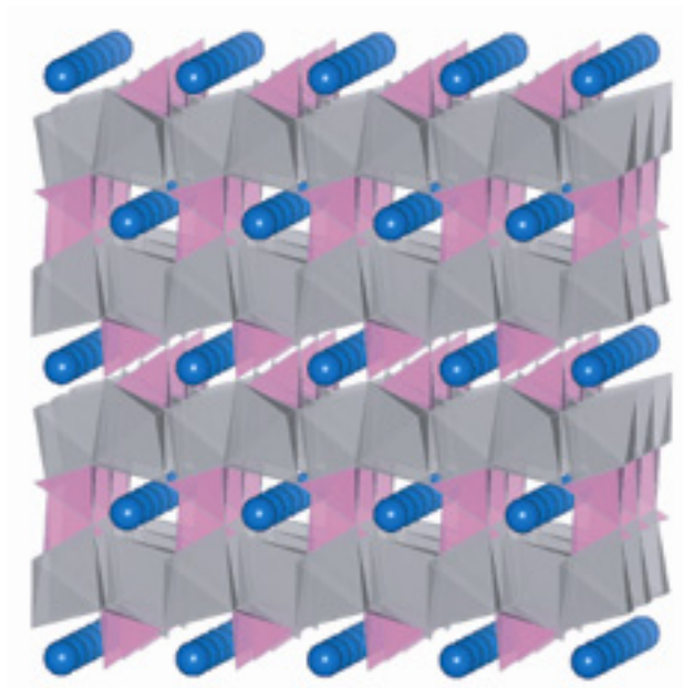
Fig. 1.6 LiFePO 4 olivine type structure.
