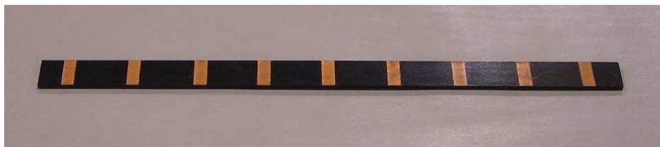
(b) Cross-ply laminate with nine electrodes
