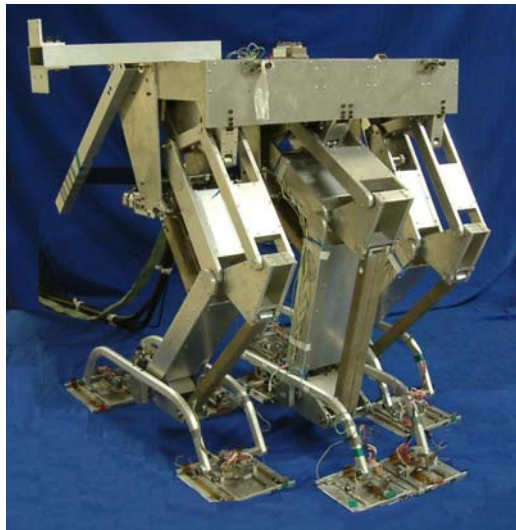
Fig. 1.4 Photo of the prototype IV (Step length:300mm, Mass:49kg, Width:760mm, Height:925mm)
