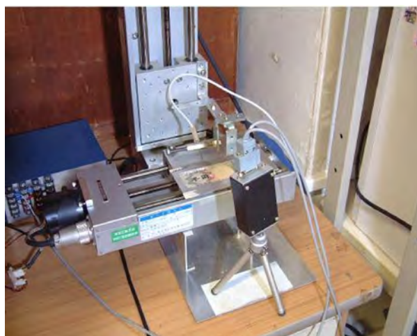
Fig. 4.3: Photograph of optical fiber feeler scanning system
