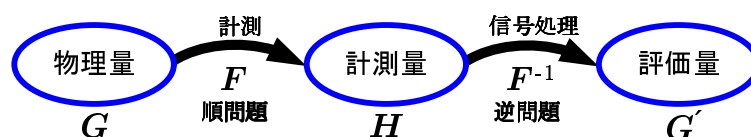
Fig. 1.3: Relation between sensing and signal processing on general inverse problem
