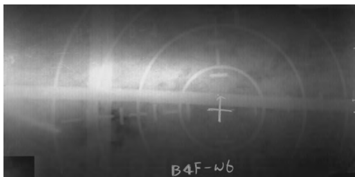
Fig. 5.24: Example of X-ray photograph of actual concrete wall
