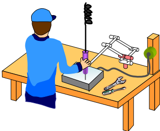
Fig. 1. Concept image of a light duty arm for a cellular manufacturing system
