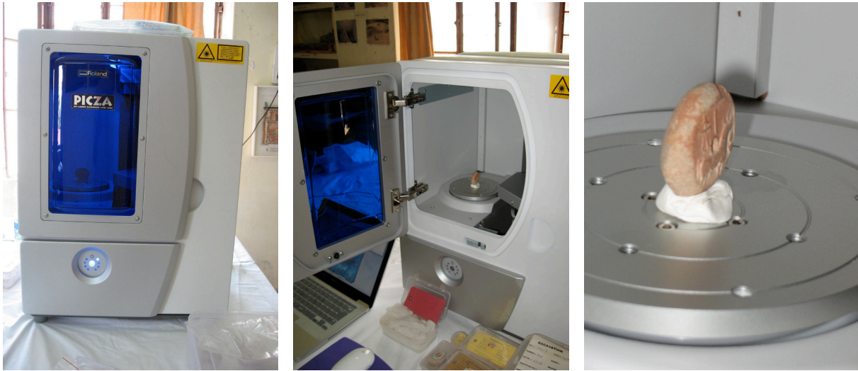
Figure 5.1.24 Roland PICZA (LPX-1200) (Left: External appearance, Center: Inside of the machine, Right: Turntable)
