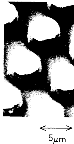
Fig. 8-3 SEM photograph of SiO 2 /TiO 2 (7pair, 5 μm φ) patterns etched by RIE system. Power: 100W, Etching gas: CF 4 , Pressure: 0.12Torr.
