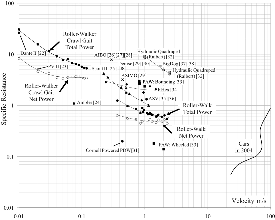
Figure 12. Velocity versus specific resistance of walking robots [22–38].
