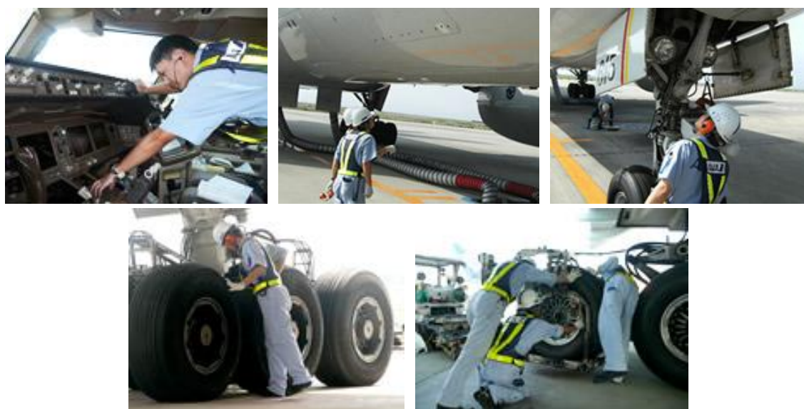
Fig. 1.10 Through flight check for commercial aircraft structures (1.14) .
