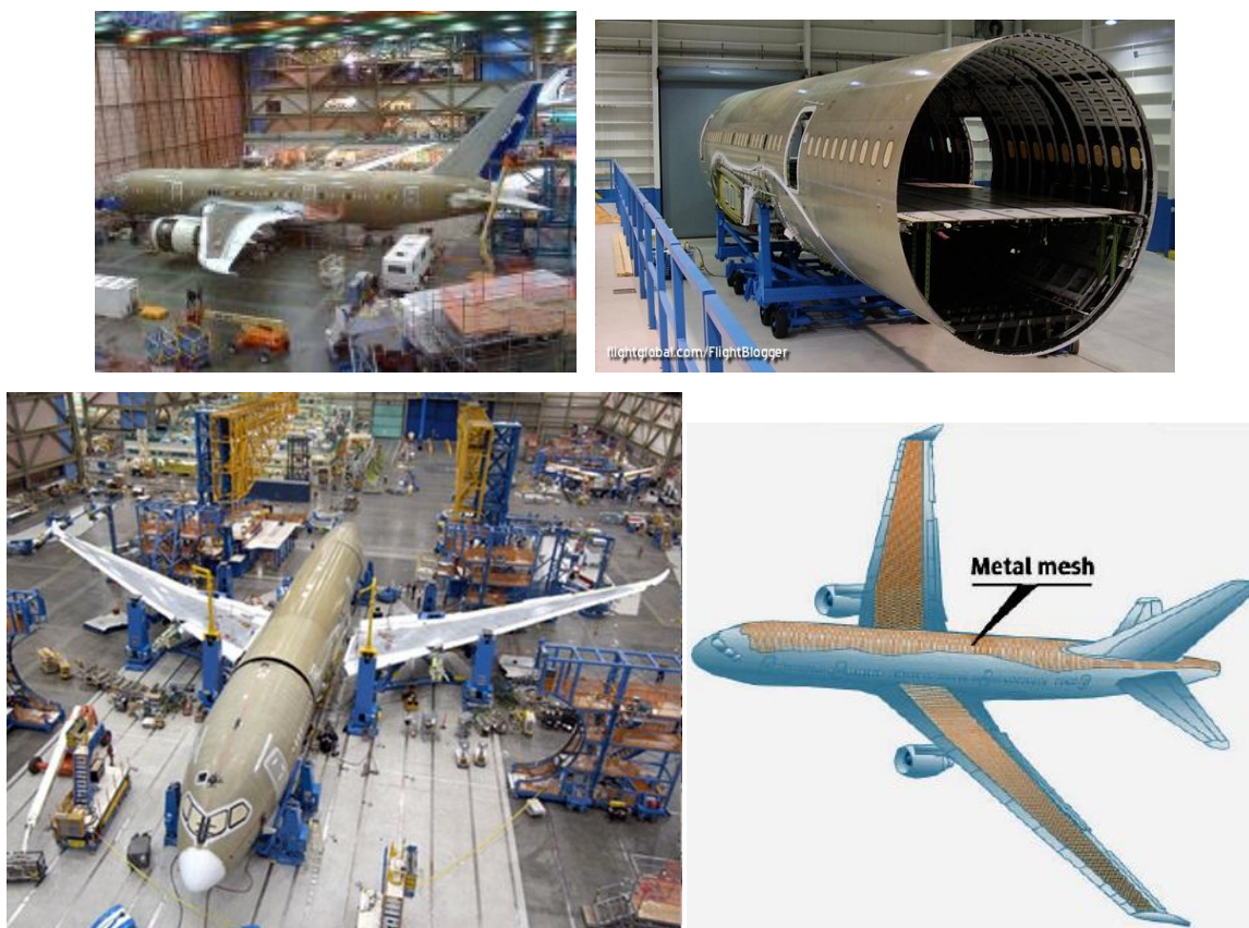
Fig. D.1 Lightning protection shield for Boeing 787 structures by acting as electrical paths for lightning strikes.
