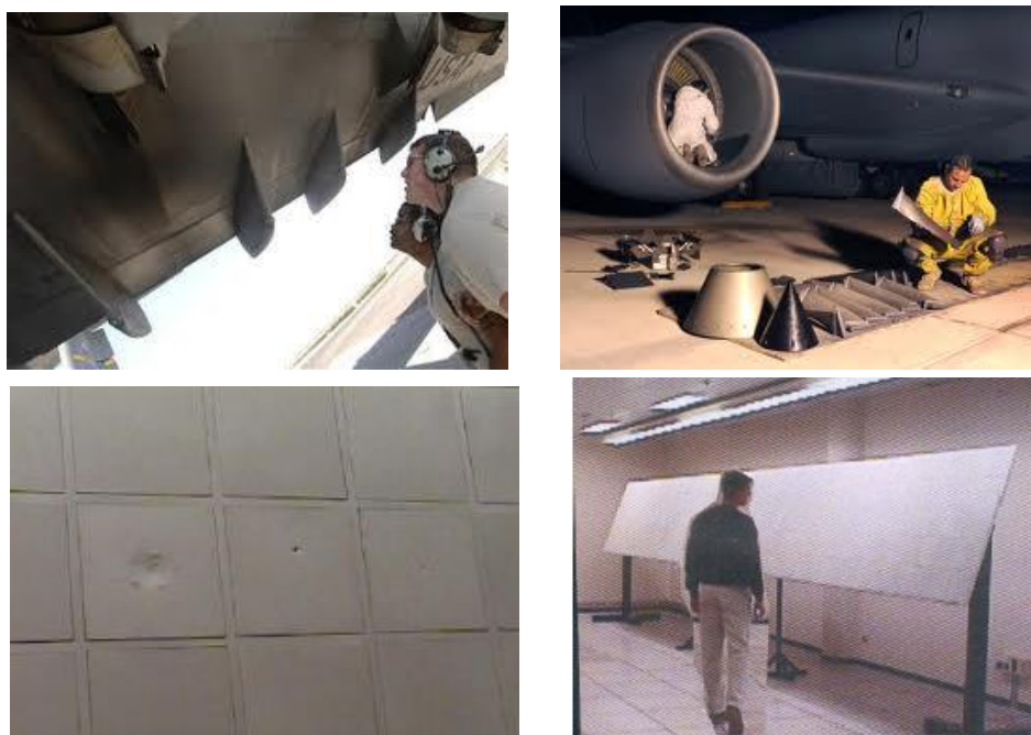
Fig. 1.14 Visual inspection for aircraft structures (1,16, 17) .
