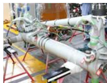
Replacement of a landing gear
