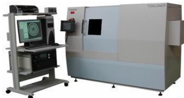
Fig. 1.18 Micro-focus X-ray computed tomography inspection equipment, TOSCANER-30000 developed by Toshiba (1,22) .
