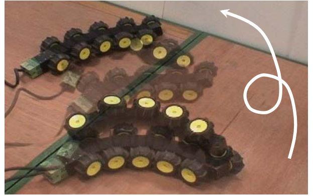
Fig. 11. Rolling over movement performed by coordinated yawing and pitching motion
