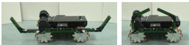
Fig. 4 Crank Wheel with bending crank-leg
