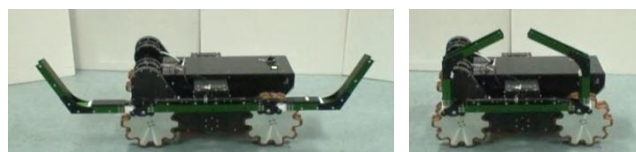
Fig. 4 Crank Wheel with bending crank-leg
