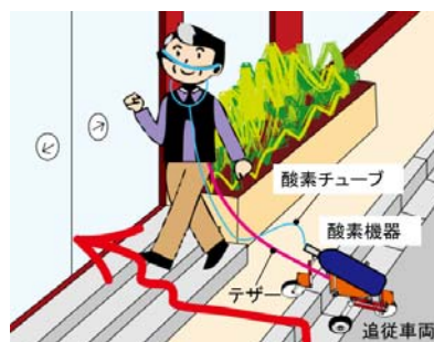
Fig. 1 Basic concept of the robotic follower carrying an oxygen tank
