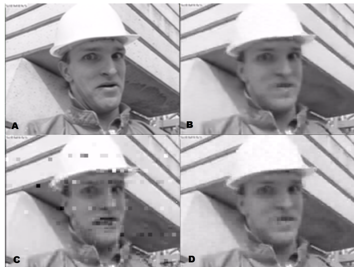
FIGURE 6.13: Comparison of the same frame. (A) Original frame. (B) Proposed multi-hypothesis feedback free system. (C) FF system. (D) Proposed single-hypothesis feedback free system. B, C and D all used the same rate.
