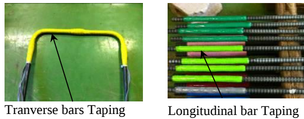
Fig. 4-2 Longitudinal and transverse bars vinyl taping
