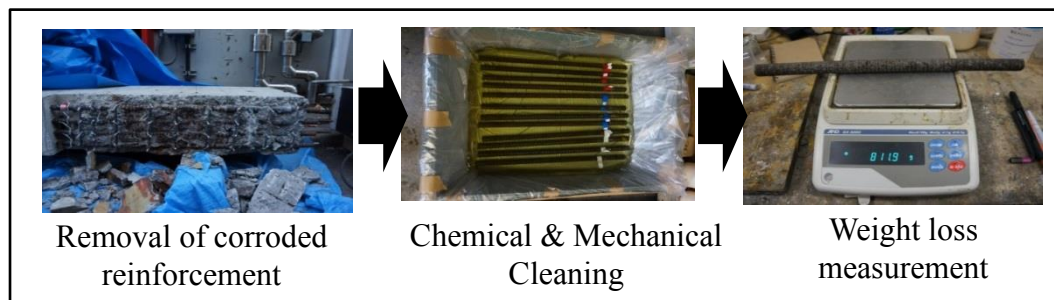
Fig. 2-4 Overview of corrosion weight loss measurement
