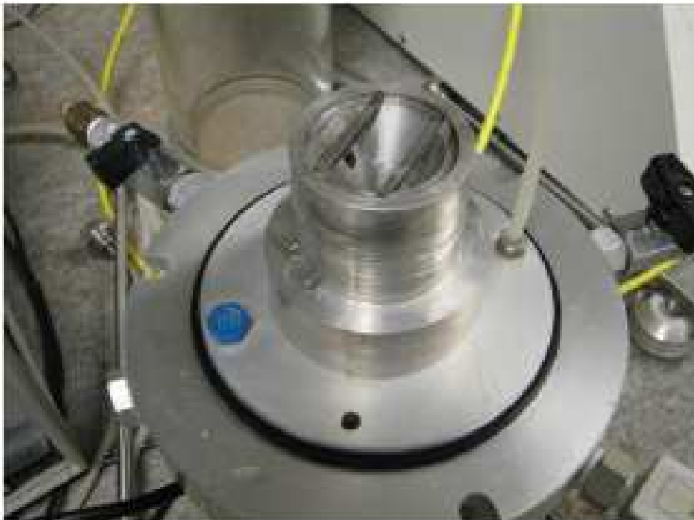
Figure 2.17 Photography of revised base pedestal (after Xiao and Shwiyhat, 2012)
