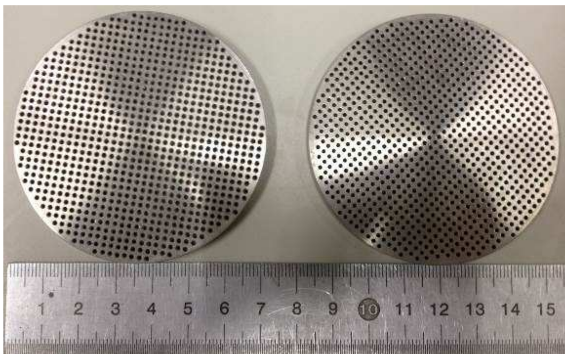
Figure 4.6 Two 5mm-thick meshes (1mm opening)
