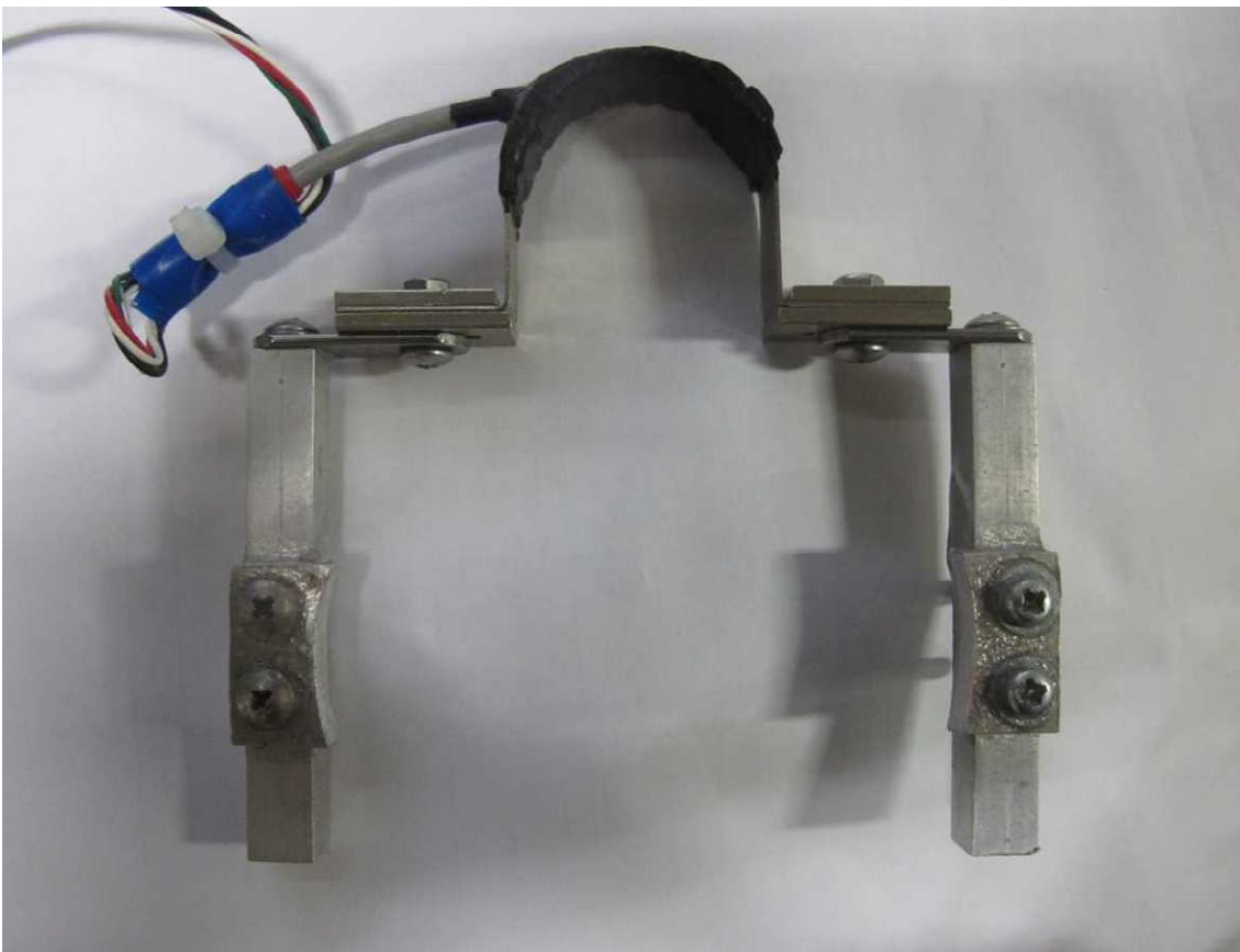
Figure 4.11 Radial Displacement Transducer (RDT)
