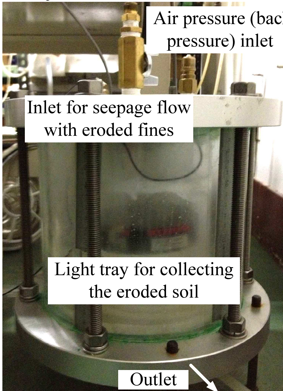
Figure 4.7 Eroded soil collection unit (sedimentation tank)
