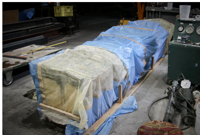
Photo 3-8 A specimen after finish casting covered with vinyl sheets
