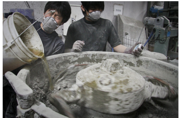
(2) Pouring water mixed with SP
