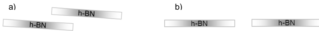
Figure 8. In-plane-oriented h-BN platelets, which is arranged a) one above the other, and b) adjacent to each other.
