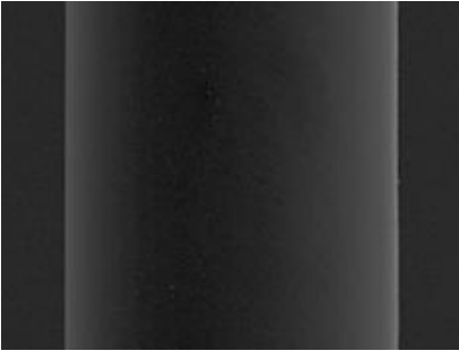
Figure 1-3. SEM photograph of smooth surface synthetic fiber produced by melt spinning.
