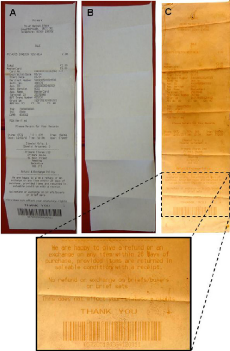
Figure 1-2 : (A) A thermal paper receipt photographed as received, then (B) following removal of the leuco dye coating with acetone and finally (C) after latent text enhancement using iodine vapor. The lower image detail illustrates the clarity and resolution obtained following iodine treatment.
