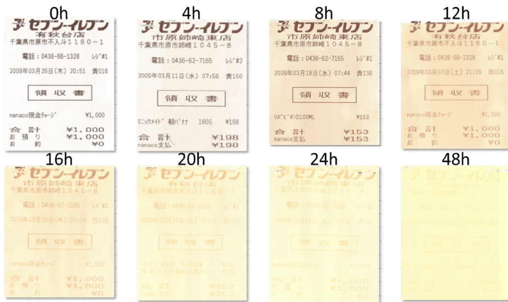
Figure 2-1: Thermosensitive paper's degradation of the look by photoirradiation. The background region turns yellow, and the image region fades by irradiation.
