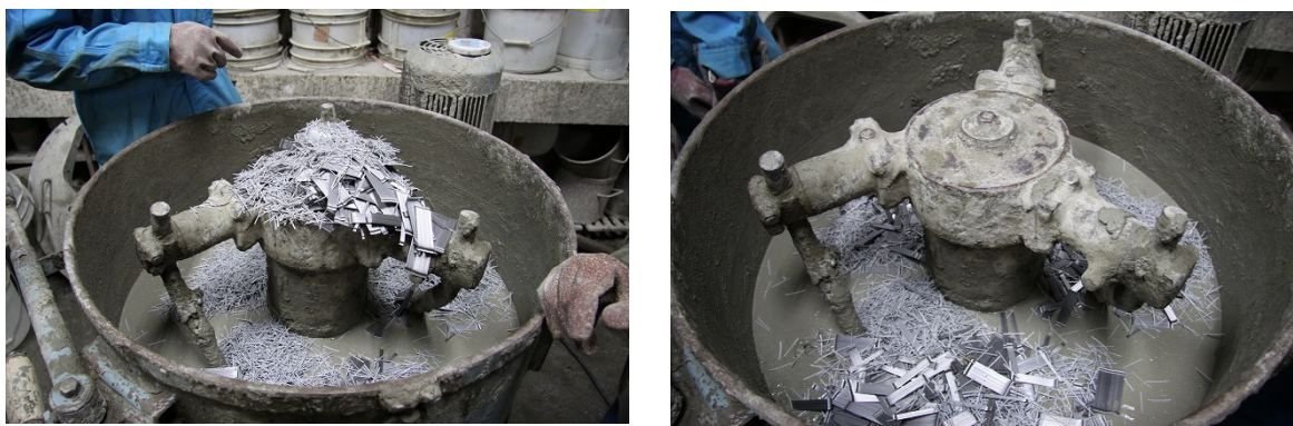
Figure 4.2 Adding fiber (Hybrid fibers between 60-mm steel and polypropylene)
