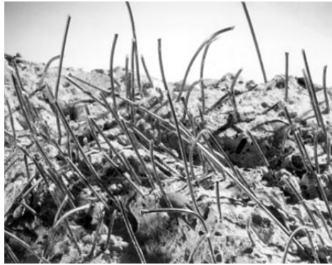
Figure 2.2 Fracture surface of FRC (ACI 544.1R-96, 2002)
