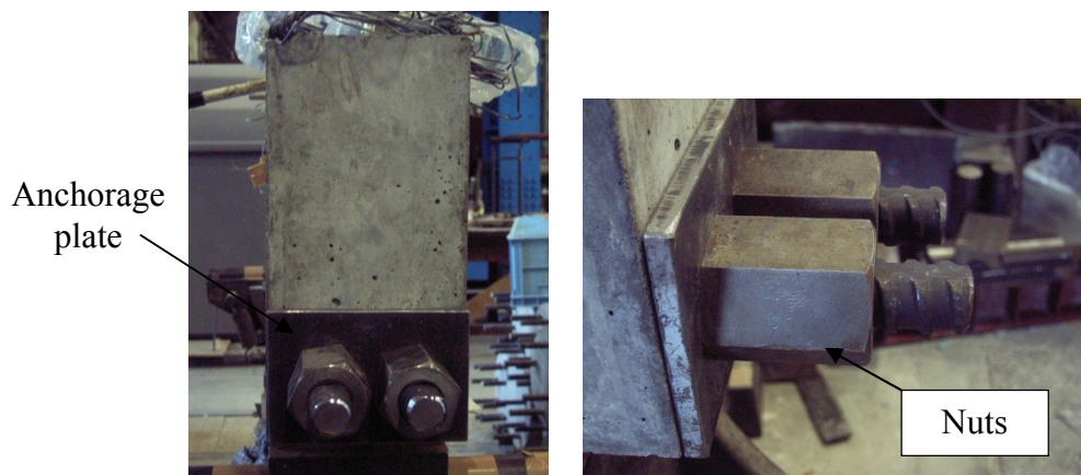
Figure 4.8 Prevention of anchorage failure
