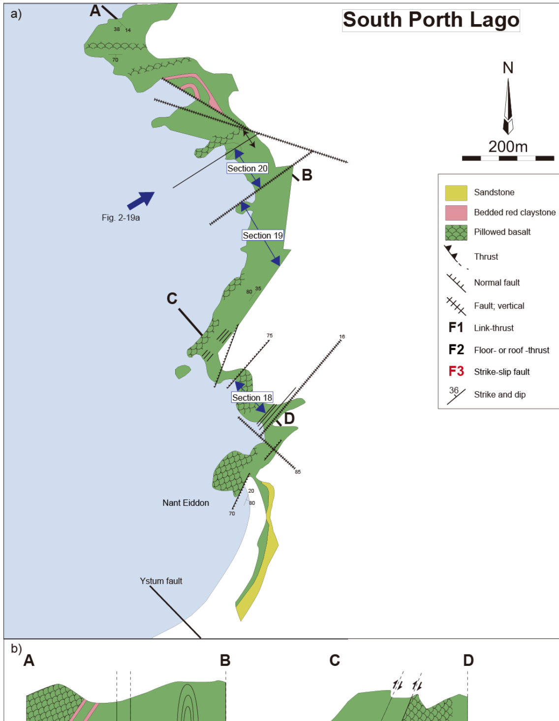
Fig. 2-18. Geologic sketch map of South Porth Lago. Note the reconstructed OPS in the middle right inset figure. Location of field photos is shown (Fig. 2-19 a). The cross section along A-B-C-D is also shown. Stratigraphic columns of section 18 to 20 are reconstructed (Fig. 2-30).
