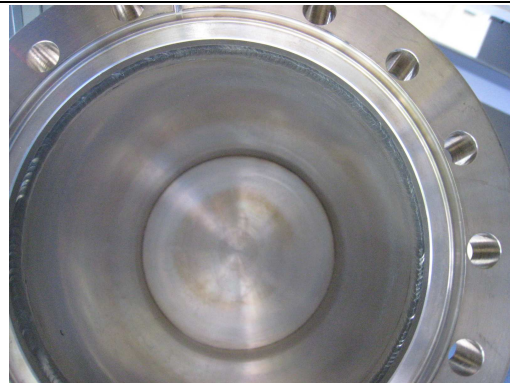
Fig.3.23 chamber's internal surfaces after dehydration (it was still clean.)
