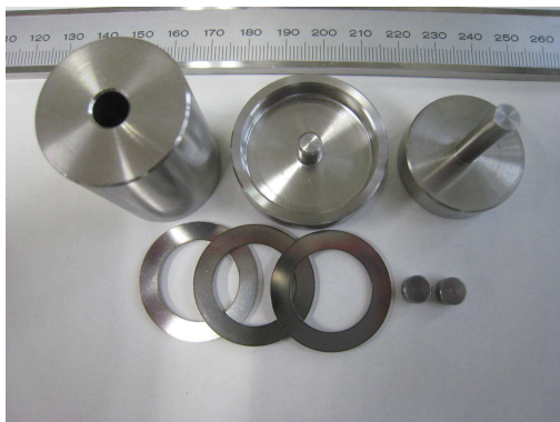
Fig. 3.15 the mold used for pellet preparation
