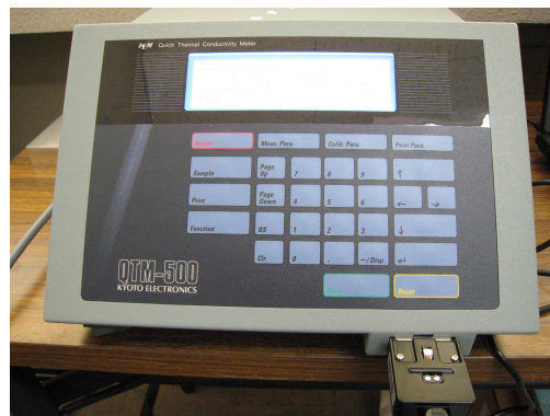
Fig. 2.3 Thermal conductivity meter (QTM-500, Kyoto Electronics)
