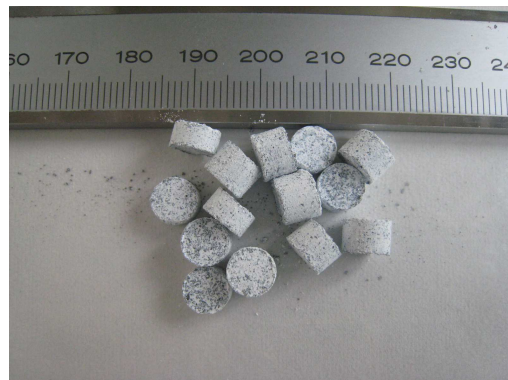
Fig. 3.16 the EM4 pellets used for the packed bed
