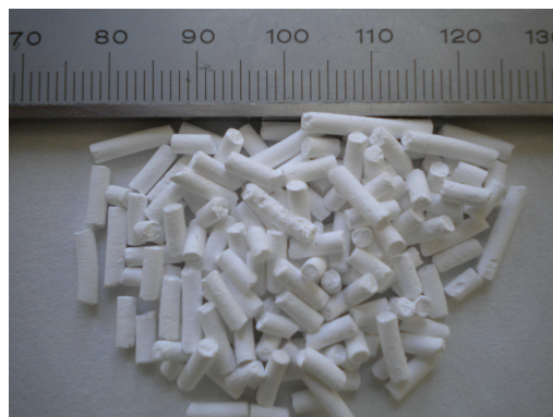
Fig. 3.1 Magnesium hydroxide pellets
