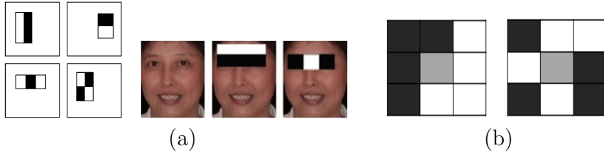
Figure 3.4: (a) are some Haar-like features shown in stick figures (left) and of real faces (right); (b) are some LBP features.
