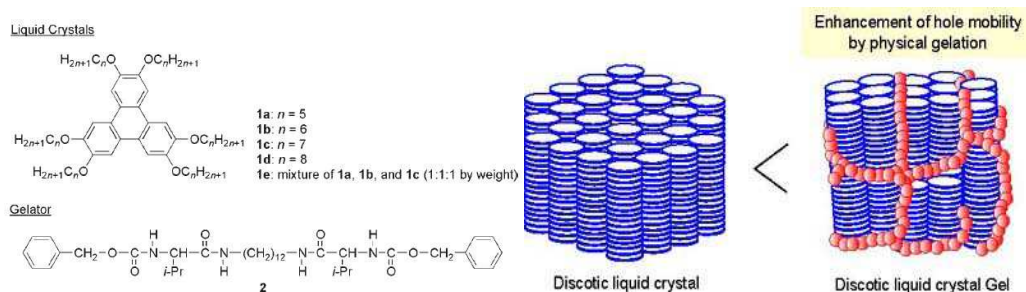
Figure 1-20 Molecular structures of discotic LC physical gels and schematic illustration of columnar structures
