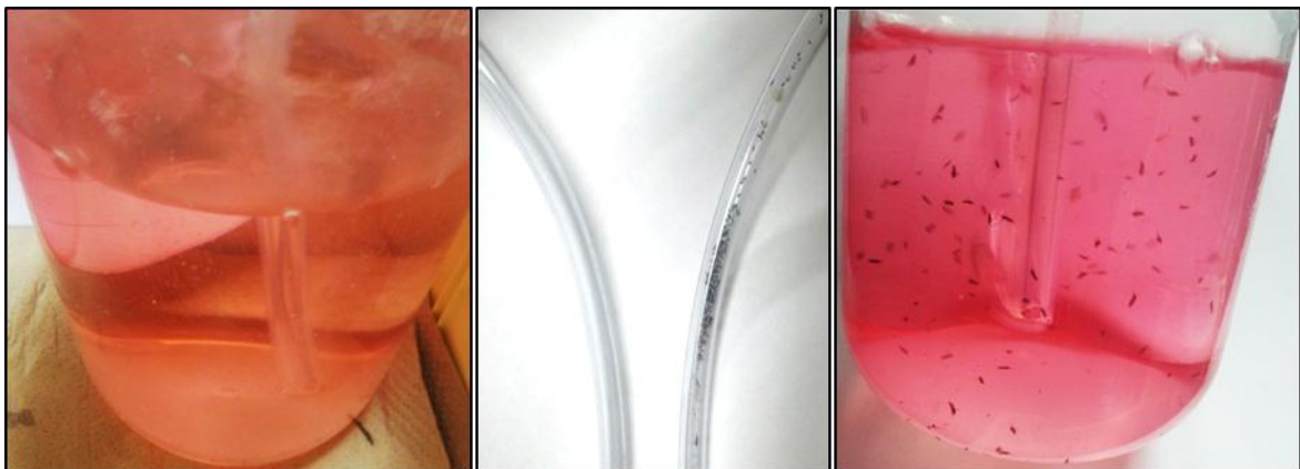
Fig.4.9. Flies and pests reaching the downstream air-supply tubes and acid traps during composting of rice straw with (left) and without (right) HTT
