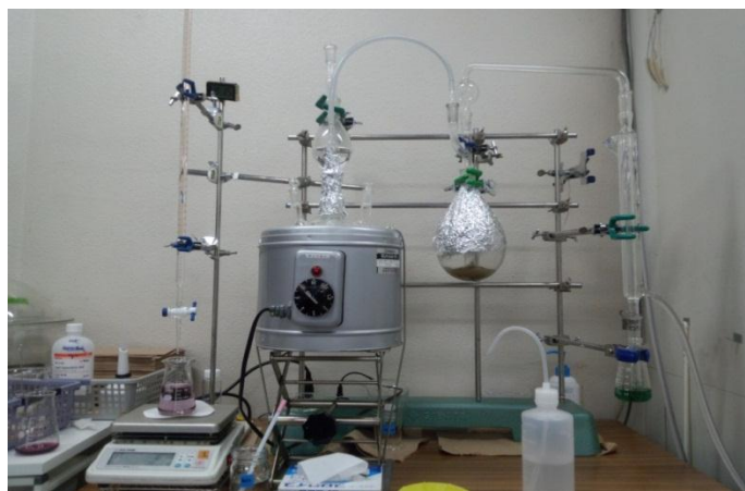
Fig.4.6. Steam distillation setup for measuring NH 4 + -N and NO 3 - -N during the experiment
