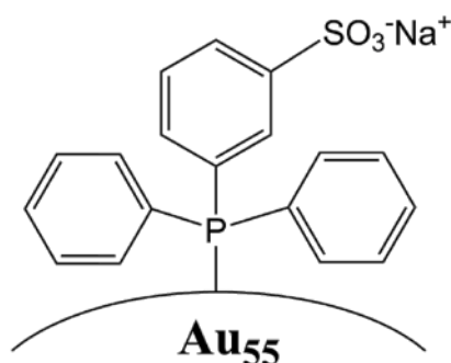
Figure 2.4 Monosulfonated triphenylphosphine ligands on \text{Au}_{55}
