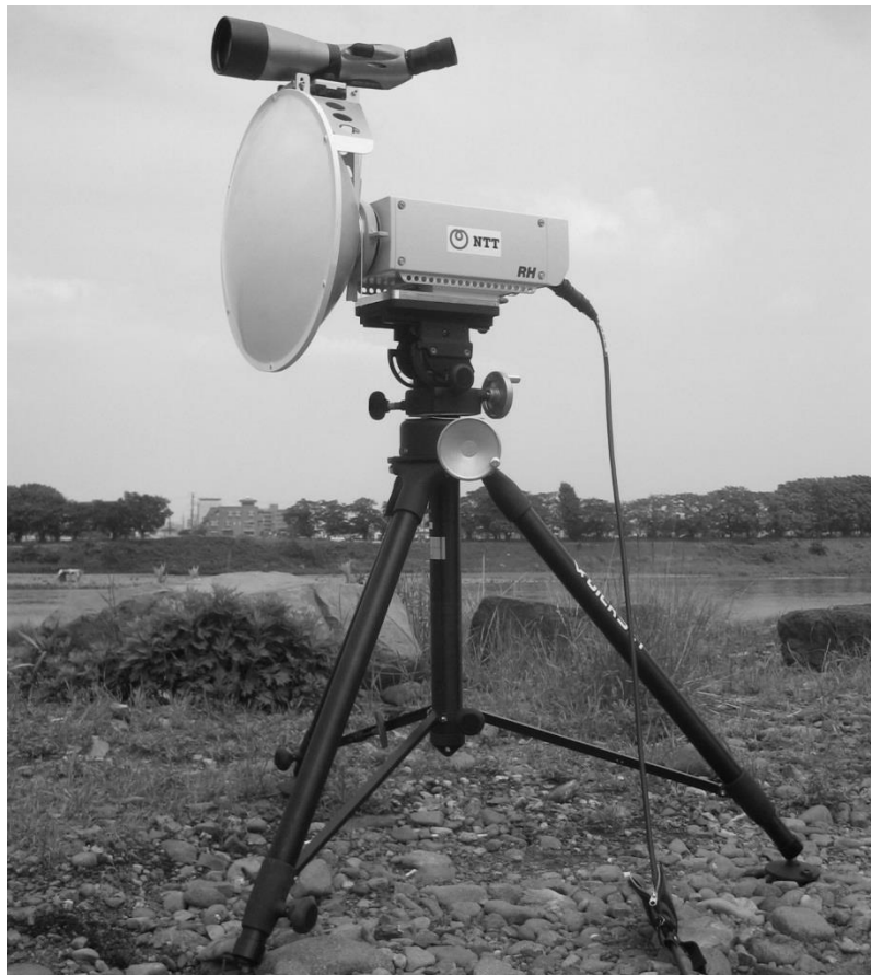
Figure 1-2. Outward appearance of 120-GHz band wireless transmitter
