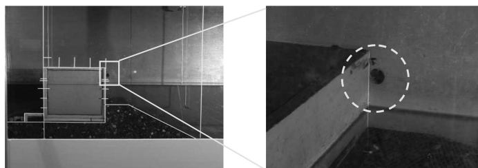
Figure 4.2 : Vent hole provided in the partition wall.
