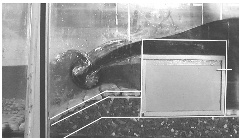
Fig. 3.7 : Snapshot of the overflow jet (Tsunami D).
