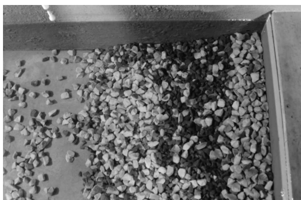
Figure 3.9 : Damage to the armor stones after Tsunami D.
