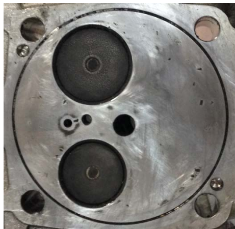
Figure 5.1 The engine head (bottom view, after the cleaning) before the engine test
