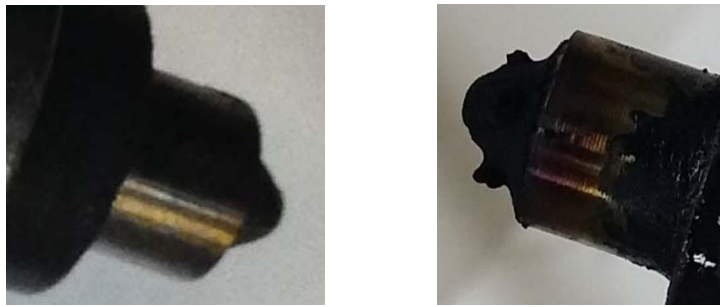
Figure 5.10 Nozzle tip after the tests: right (the diesel) and left (the 30% blend)
