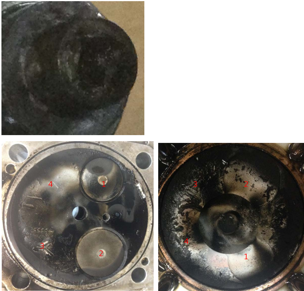
Figure 5.17 Nozzle tip, bottom view of the engine head and upper view of the piston after the engine test of the 20% blend oil
