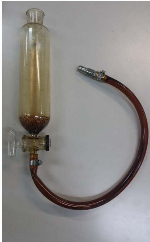
Figure 5.13 Fuel vessel and fuel tube line after the engine tests: the 30% blend
