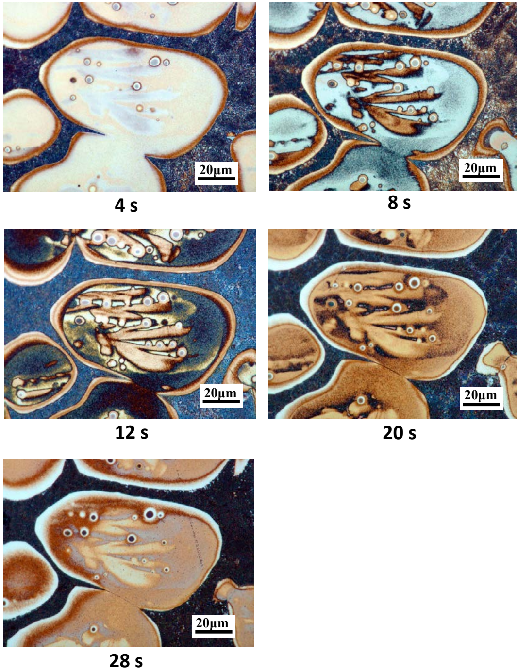
Fig. 5-9. Microstructures of Ti-contained A356 Al alloy obtained after different times of etching using Weck's reagent.
