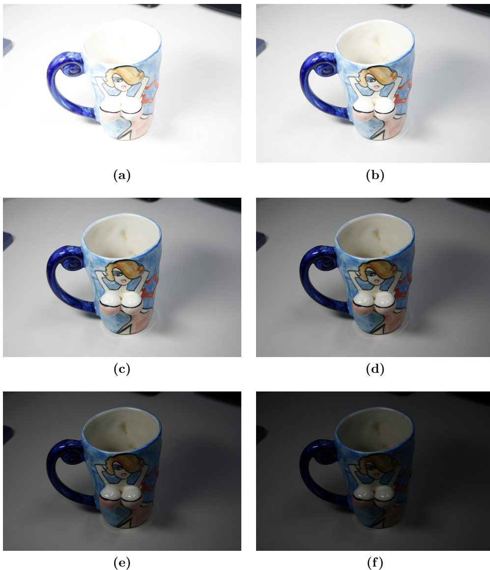
Figure 2.1: A “cup” scene used to recover the camera response curve (Canon TM EOS 300D).
