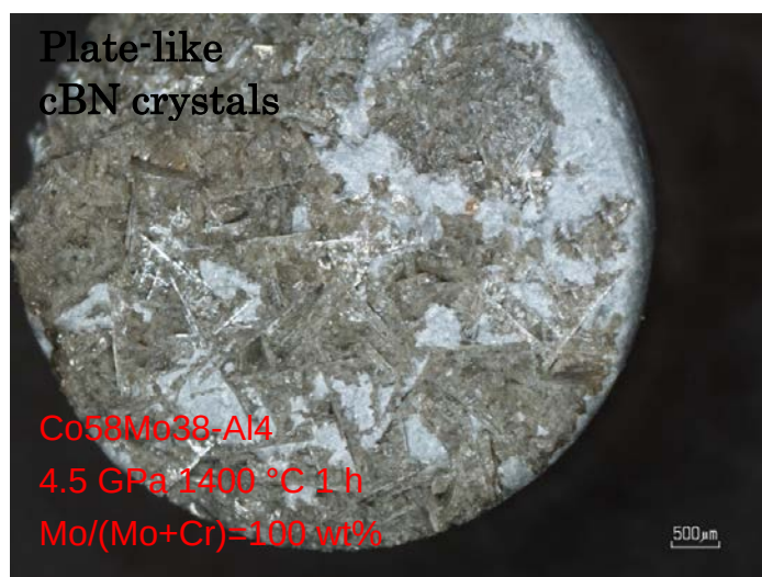
Fig. 3.12. The morphology of cBN crystals reacted at 4.2-4.5 GPa and 1300-1400 °C 1 h. with various Mo content.
