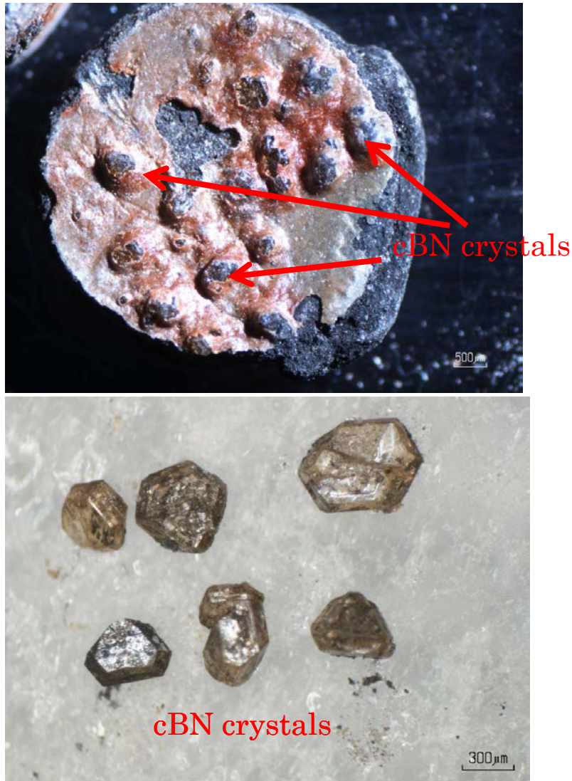
Fig. 3.7. Optical photograph of cBN synthesized using Fe 52.5 Ni 5.8 -Cr 38.8 -Al 2.9 solvent at 4 GPa 1350 °C 0.5 h.
