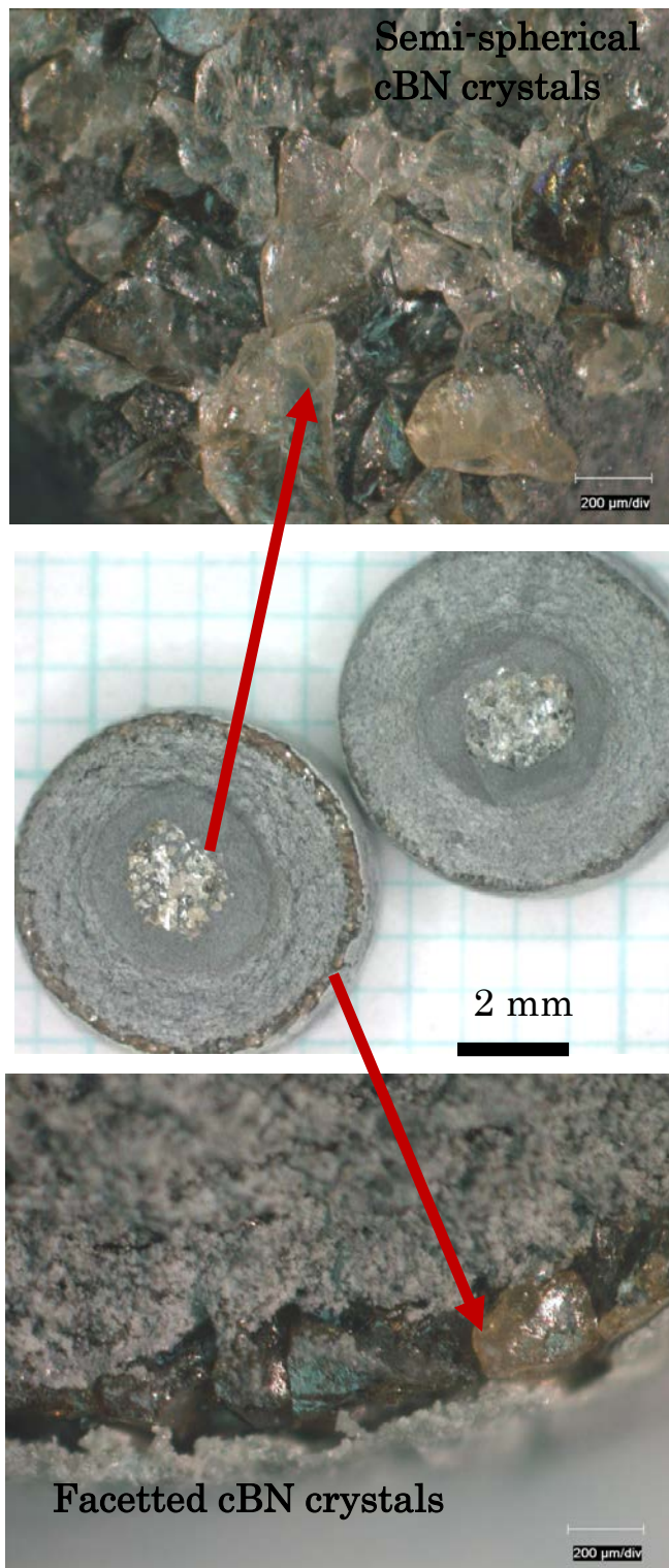
Fig. 3.8. Optical photograph of cBN synthesized using Fe 52.5 Ni 5.8 -Cr 38.8 -Al 2.9 solvent at 4.2 GPa 1280 °C 0.5 h.
