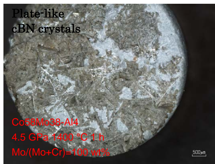
Fig. 3.12. The morphology of cBN crystals reacted at 4.2-4.5 GPa and 1300-1400 °C 1 h. with various Mo content.
